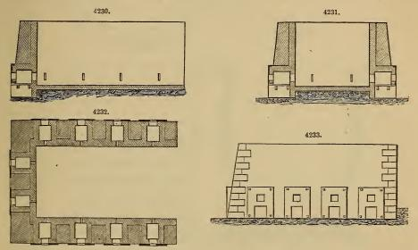
able, on the ground that combustion is slower in the angles than in the centre. If the heat be regulated to properly calcine the centre of the mass, the stone lying in the angles will scarcely have altered from its raw state.
